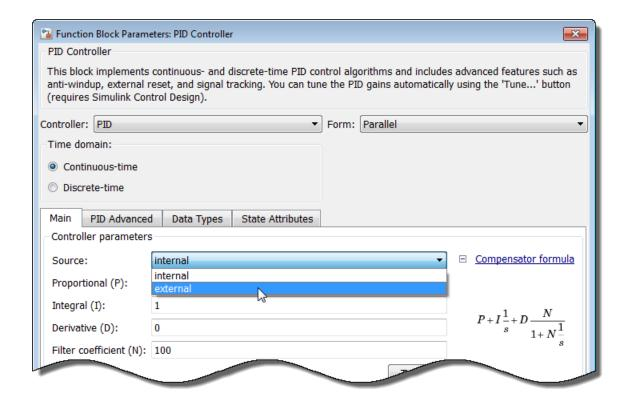
When you click **OK** or **Apply**, the new inputs appear on the block in the Simulink model.
